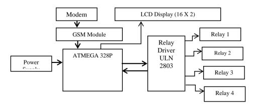
Fig. 1. Block diagram of Appliances Control.
